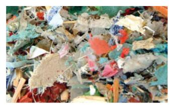
Left, used tires are chipped and used as an alternative fuel in cement kilns, helping to reduce landfill Right, Refusederived fuel is made from treated household and commercial waste
